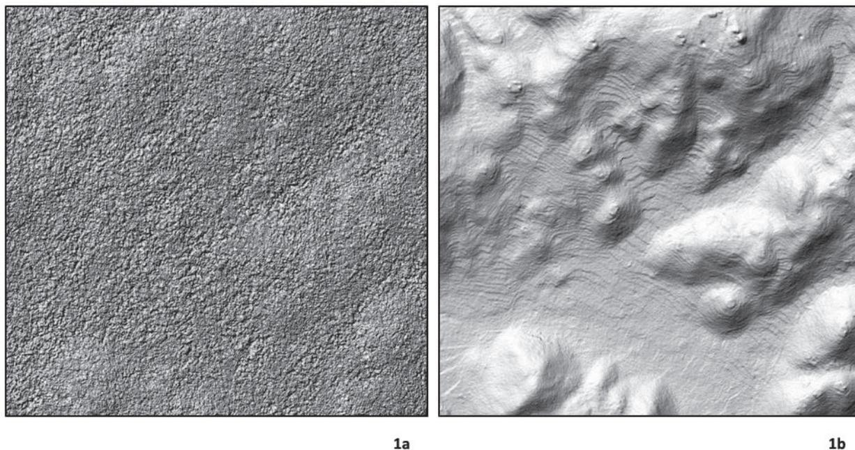
**FIGURE 1.** Examples of two DEMs: (a) Digital Surface Model (DSM) of tree canopy overlying the Caracol's Puchituk Terminus; (b) Digital Terrain Model (DTM) showing the bare earth visualization of Caracol's Puchituk Terminus.
