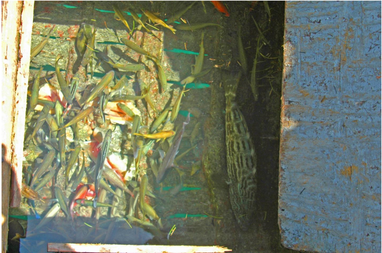
Figure 10: Live well of the fishing boat " Lively Hope ", showing live fish from a four-day fishing expedition. Note the slats in the bottom of the hold to allow for water exchange. Photo courtesy of David Smith.
